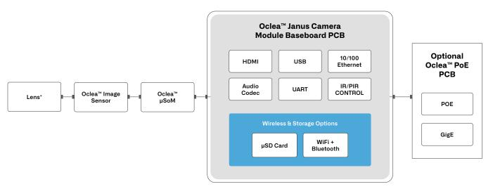
$^{\ast}$  Lens is not included in the Janus Camera Module package
